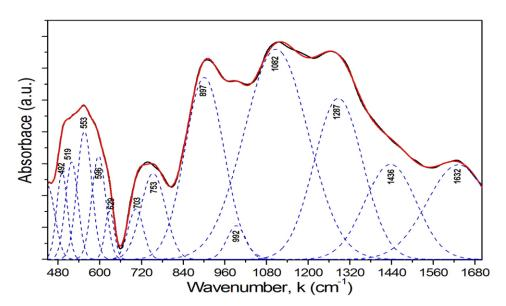
Figure 2: The band deconvolution of FT-IR spectra for glass of 2% CuO content in the spectral
