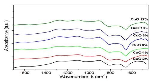
Figure 1: FTIR absorbance spectra of CuO nanopowders doped with barium phosphate glass
